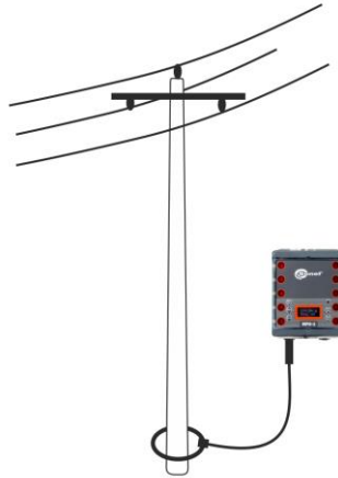
Fig.9. Operating the device with single clamps
